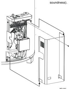
Figure 7 - Taking off and mounting the column
