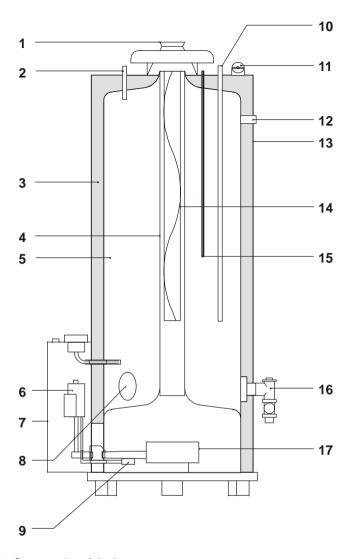
Figure 1 - Cross section of the heater
